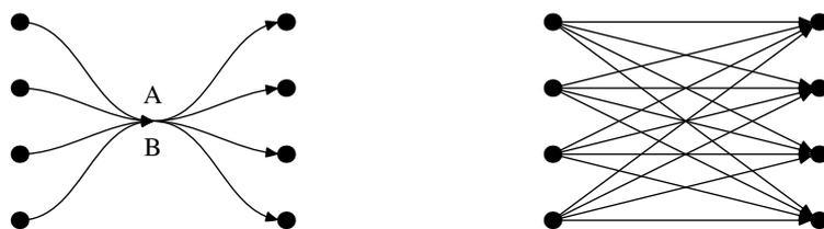
**Figure 6.** The cost of the gadgets for equations of the form  $x + y + z = 1$  is lowered by the above transformation. The figure to the left shows the connection between two such gadgets as it is obtained by joining B in one gadget as shown in Fig. 2 with A in another such gadget. The figure to the right shows how this connection is actually implemented.
